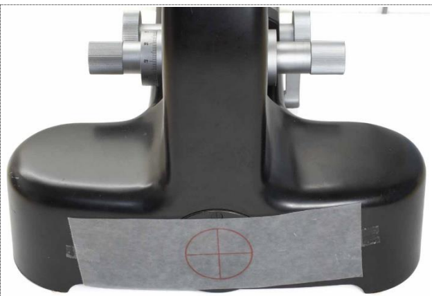
Figure 18: The lamphouse port symmetrically covered with the collimation target wax paper printout.
